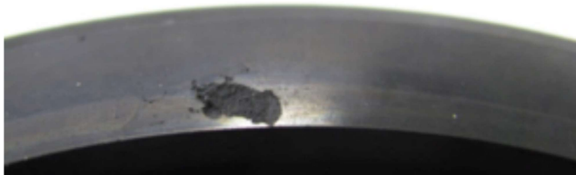
Example of a carbon blister caused by improper barrier fluid selection
