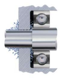
Without a viable bearing protection device installed, contaminants such as water, corrosive liquids, and dust/dirt can enter the bearings on pumps and electric motors. Costly bearing failures, motor rewindings, and production downtime are the result.
