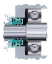
By installing Bearing Gard II bearing protection, bearing life can be increased to extend equipment MTBF. Bearing Gard II bearing protection is easy to install and on most equipment requires no modification. Electric motor bell housings typically require a standard machining retrofit common at most motor rebuild shops.
